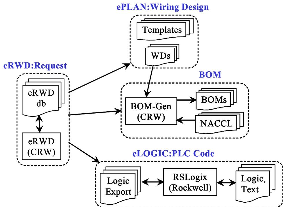
CCRW's ePLAN and eLOGIC Automatically Generate H/W Design, BOM, and Control Code
